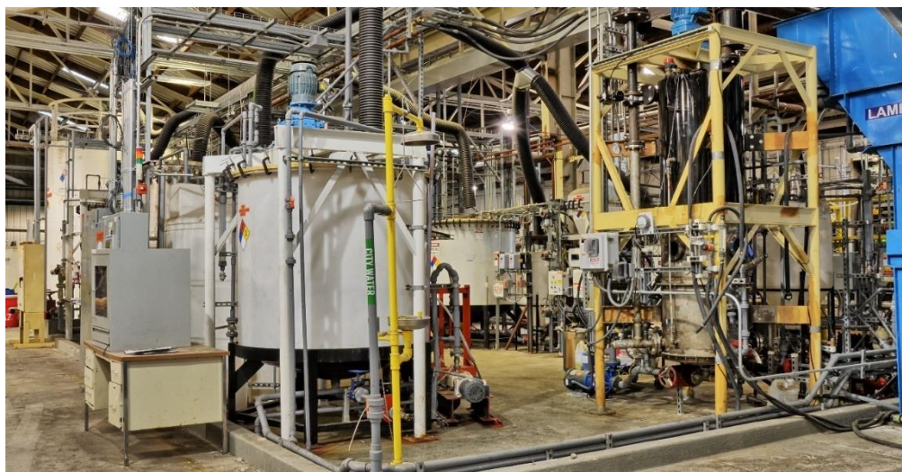
Figure 2. CaCO 3 cement pilot plant.
