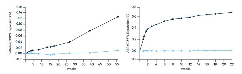
VC³ cements demonstrate exceptional longterm durability. Expansion due to sulfate attack or alkali-silica reaction (ASR) is eliminated.
