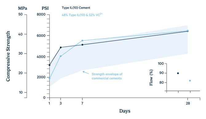
The vaterite-calcined clay pre-blend allows clinker cut < 50% and increases early-age strength.
