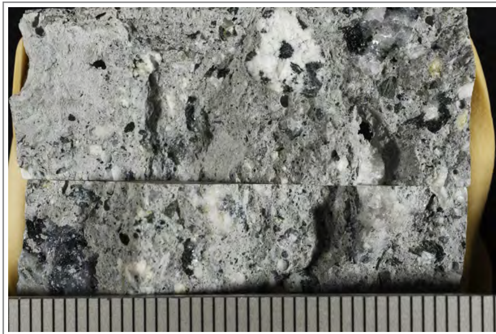
Figure A9. Photograph showing detail of the paste on freshly fractured surfaces. Scale is in millimeters.
