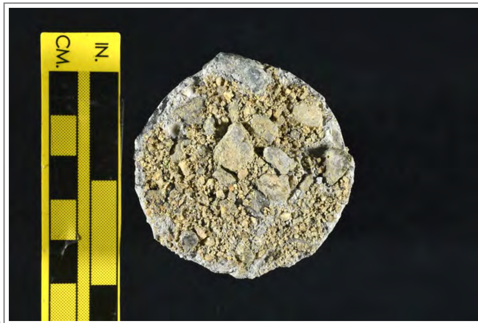
Figure A1 (cont'd). Photographs of the core in as-received condition showing (c) the side of the core and (d) the bottom surface of the core. The yellow scale is ~ 150 mm (6 in.) long; the small and large divisions are in centimeters and inches, respectively.
