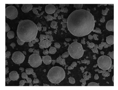
Binder based on the transformation of vaterite to aragonite or calcite, which has been successfully utilized to manufacture building materials.
