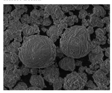
Fineness and morphology are designed to increase packing efficiency, accelerate cement hydration, and improve workability.
