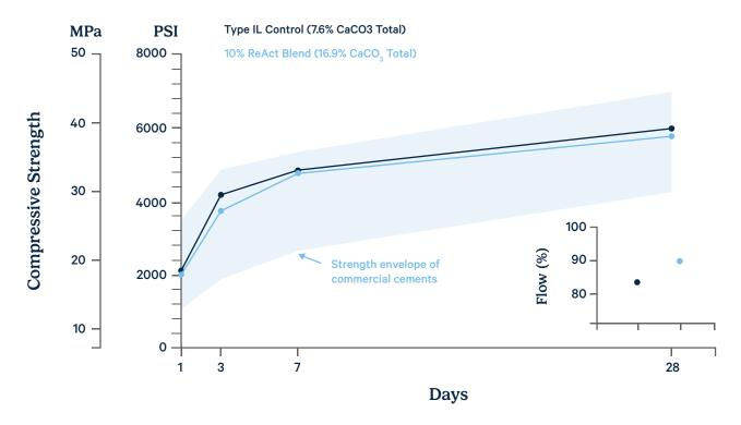
10% ReAct Blend enables the further clinker reductions, while maintaining strength and improving flow.
